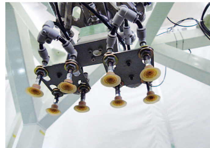
Double gripper for handling packages
