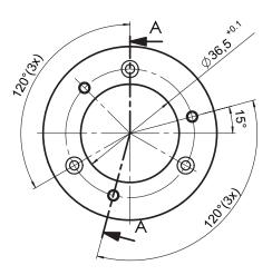
Order code 8.0010.2230.0000 (Set) Includes flange and screws for encoder mounting.
