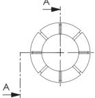
Isolation inserts prevent currents from passing through the encoder bearings. These currents can occur when using inverter controlled three-phase or AC vector motors and considerably shorten the service life of the encoder bearings.
