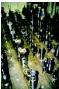
Tool handling in the machining center tool magazine with BIS C data carriers. Application at MTU Friedrichshafen.
