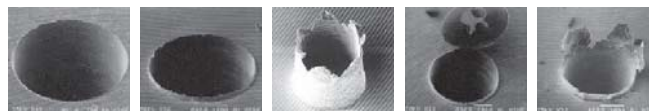
Type 1 Type 2 Type 3 Type 4 Type 5 Classification for burrs at the bore exit according to height and form
